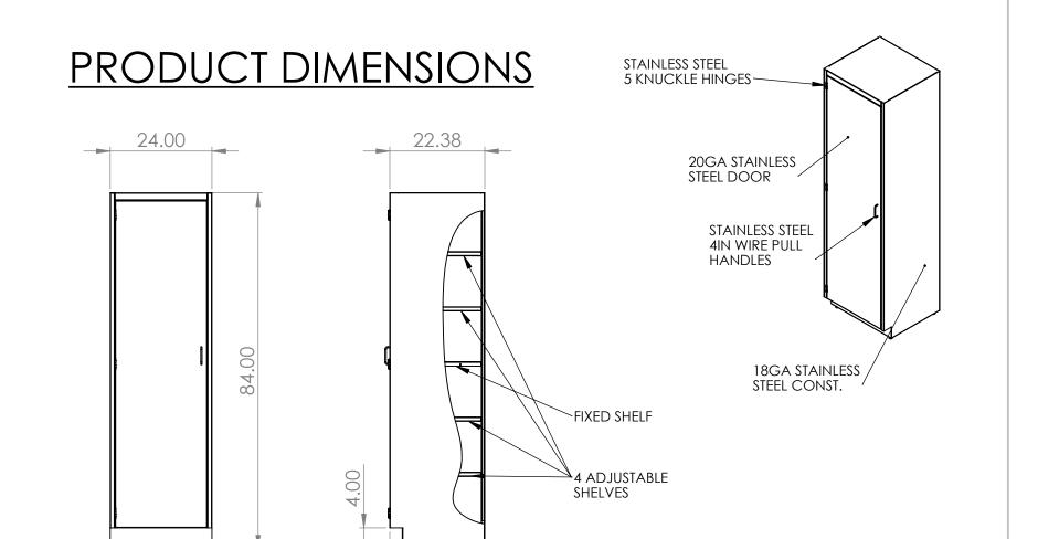
ADJUSTABLE/REMOVEABLE RUBBER BOTTOM FOOT
