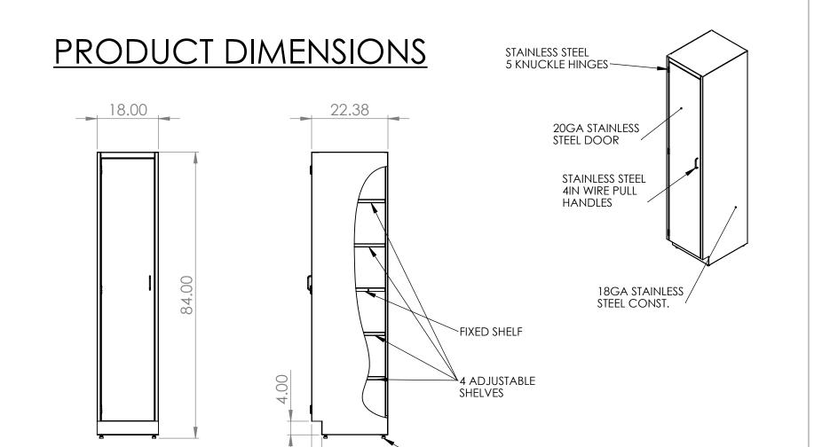
ADJUSTABLE/REMOVEABLE RUBBER BOTTOM FOOT
