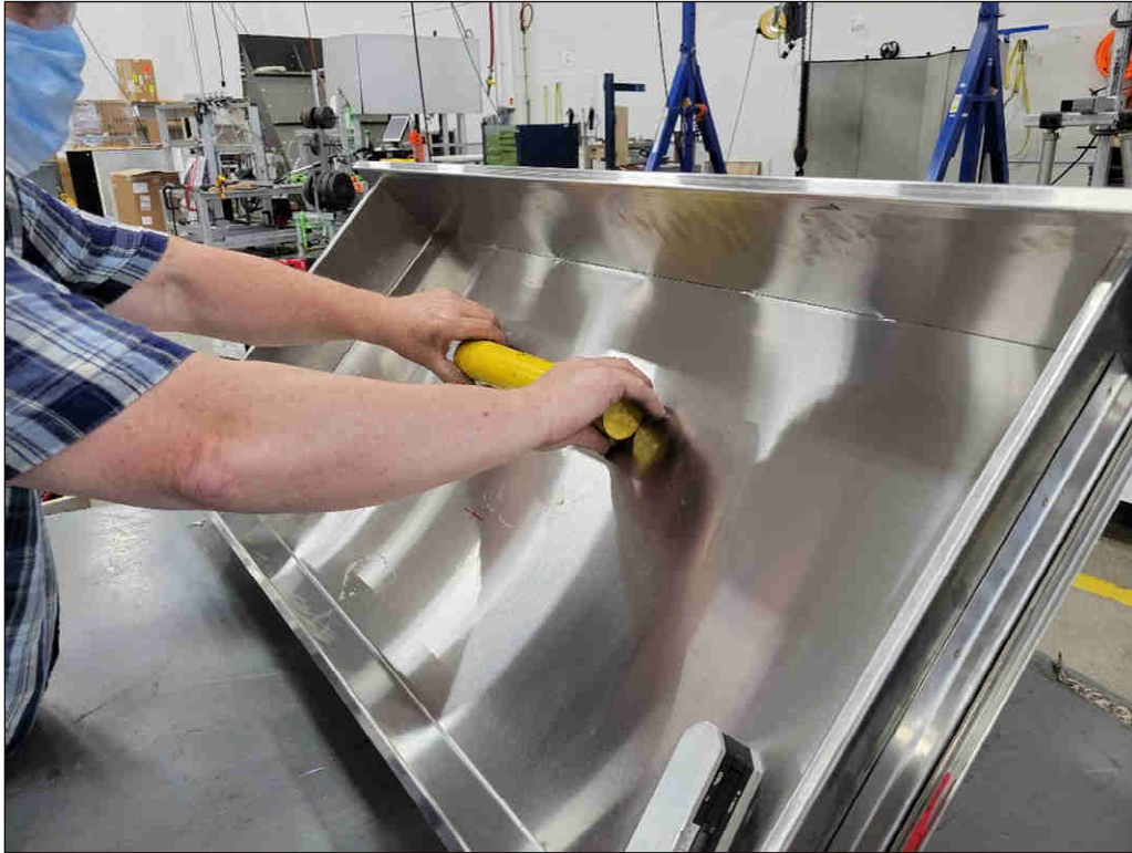
Drawer Internal Rolling Impact Test – Front to Rear
