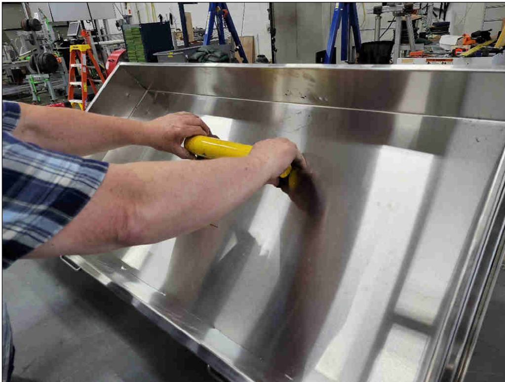
Drawer Internal Rolling Impact Test – Rear to Front
